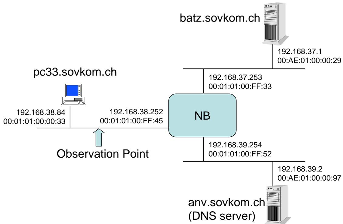
Figure 2: The network of Problem 1, with NB configured as router
